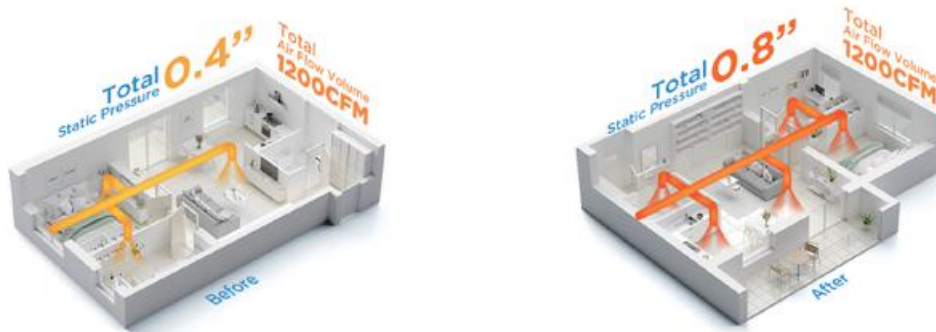
Different Ductwork Designs, Same Air Volume
